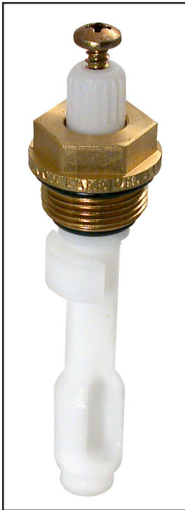
60-4D-0 PLASTIC For Phoenix 3 valve wall mount tub/shower diverters. Used in wall thicknesses up to 7/8". Old style, obsolete in 1991, not interchangeable with 639-5-0.
